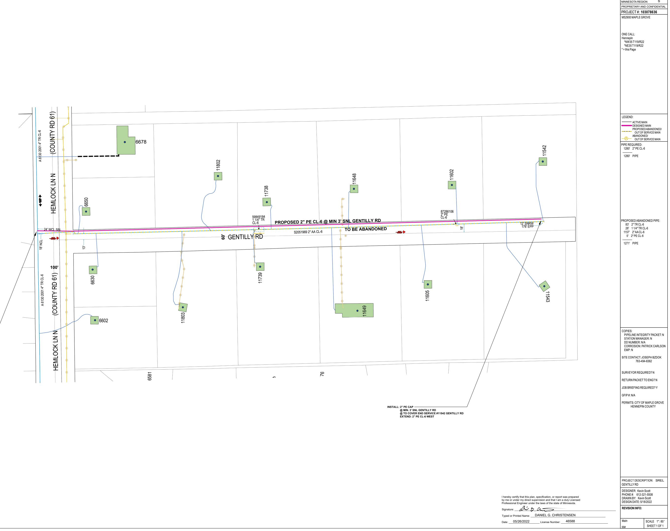
EXISTING: 4" PE TEE (A61302001) -18' NCL GENTILLY 24' WCL SBL COR RD 61 EXISTING: 4X2 PE REDUCER (A61302001) 18' NCL GENTILLY LA 24' WCL CO RD 16 INSTALL: 4X2 HVPT @ MIN. 3' SNL GENTILLY RD EXTEND: 2" PE CL-6 EAST
