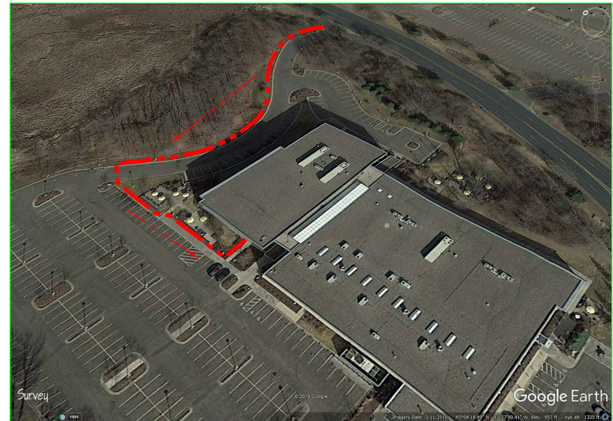
FIBER ROUTE ALONG NORTHSIDE OF DRIVEWAY GOING WEST THEN GOING SOUTH ALONG PARKING LOT AND TO THE BUILDING
