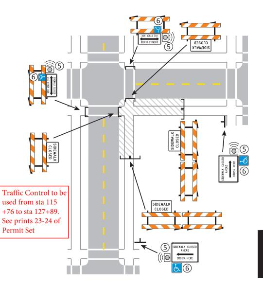
ALTERNATE PEDESTRIAN ROUTE CROSSWALK CLOSURES AND PEDESTRIAN DETOURS 3 DAYS or LESS LAYOUT 88b LAYOUT 88a & b 6K-88b
